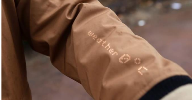
Figure 7 Smart clothing that is electrically conductive embedding a Temperature sensor with a display screen on a winter jacket (Image Source: Thread in Motion)
