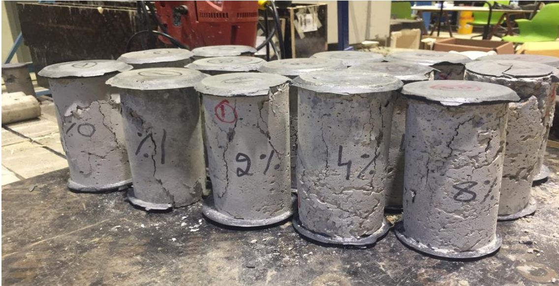
Figure 12. Failure of samples after compressive strength test
