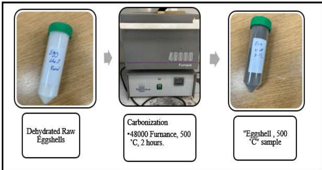
Figure 3.4: Carbonized Eggshells (CES) Adsorbent Preparation
