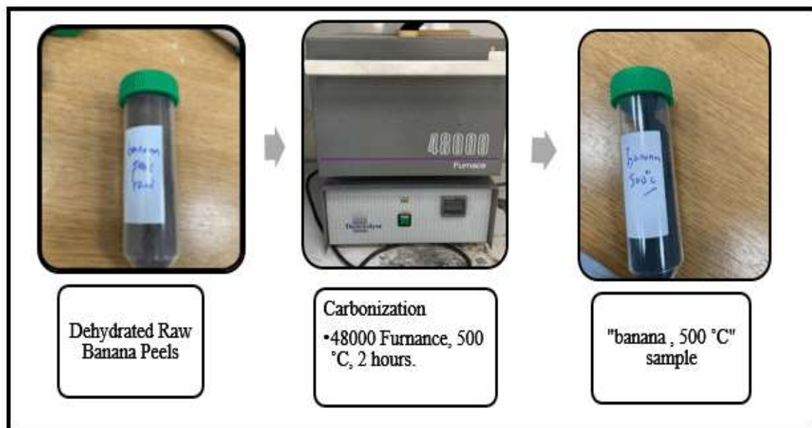
Figure 3.2: Carbonized Banana Peels (CBP) Adsorbents Preparation
