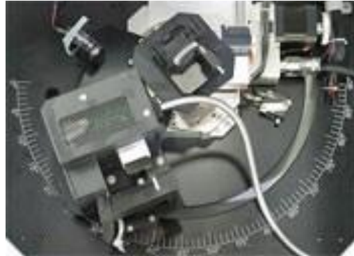
Figure 64: figure showing the adjustment of the container ARN 915 Mode used for reflectance measurements [185]
