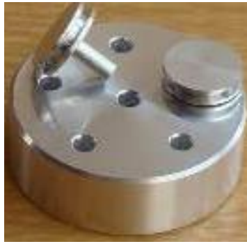
Figure 52: figure showing sample holder and stabs on which the sample is attached used in SEMs [199]
