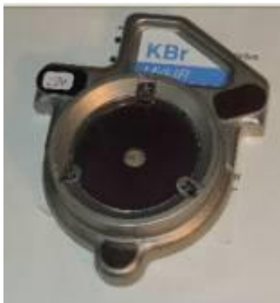
Figure 95: figure showing the KBr beam splitter used in our FTIR system [180]
