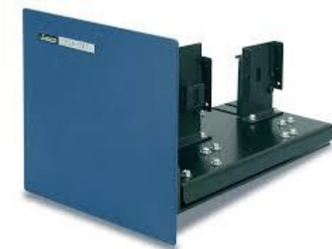
Figure 63: figure showing sample holder for solids used in our UV-VIS transmittance measurements [185]
