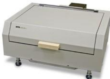
Figure 61: Figure showing our Reflection measurement apparatus that attaches to our UV-VIS-NIR spectrophotometer [185]
