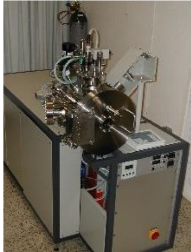
Figure 22: figure showing our pulsed laser deposition [199]
