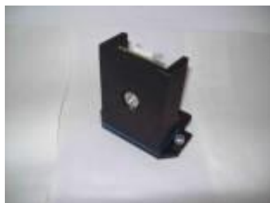
Figure 97: figure showing the DTGS-KBr detector used in our system [180]
