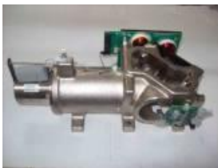
Figure 96: figure depicting the Michelson interferometer attached to our FTIR [180]
