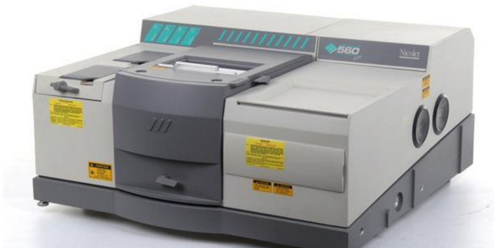
Figure 93: figure showing our FTIR system [180]
