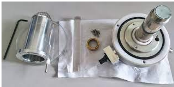
Figure 47: figure showing the Everhart-Thornley detector set up [87]
