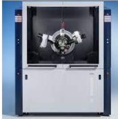
Figure 29: figure showing our Bruker AXS D-8 Advance Bragg Brentano diffractometer [129, 199]
