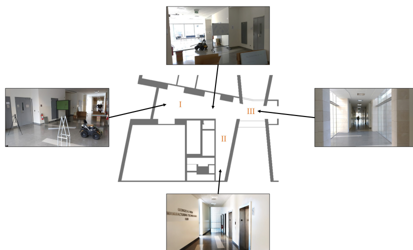
Figure 3.14: Blueprint of the testing arena and photos of the experimental setup. Region I contains obstacles higher/lower than the LiDAR's detection plane, glass walls, and reflective objects. Region II is a corridor with poorly textured walls, and Region III has two glass walls facing each other. The robot starts in Region I and cannot traverse to Regions II and III since the exit is narrow.
