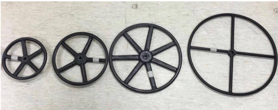
Figure 3: The four handwheels used in the study, with respective diameters of 35, 45, 60, and 70 cm.
