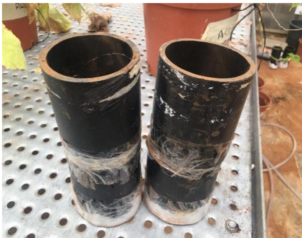
Figure 17. Columns filled with 2 soil types
