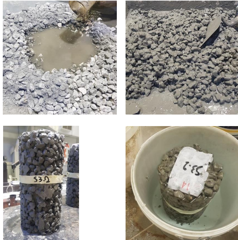
Figure 12: Pervious concrete sample preparations from mixing materials to curing for specimen using 9.5 mm BA as 20% aggregate replacement
