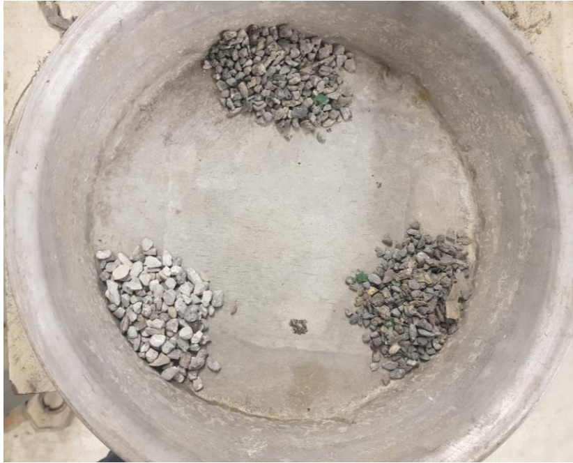
Figure 7: Difference between non-sorted (right), semi-sorted (top) and sorted (left) aggregates
