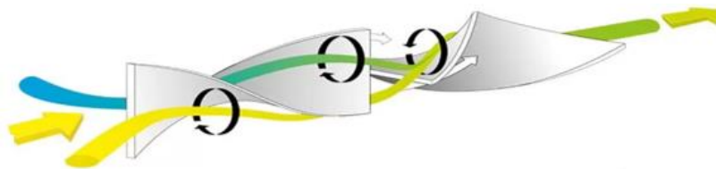
Figure 2 Kenics flow pattern
