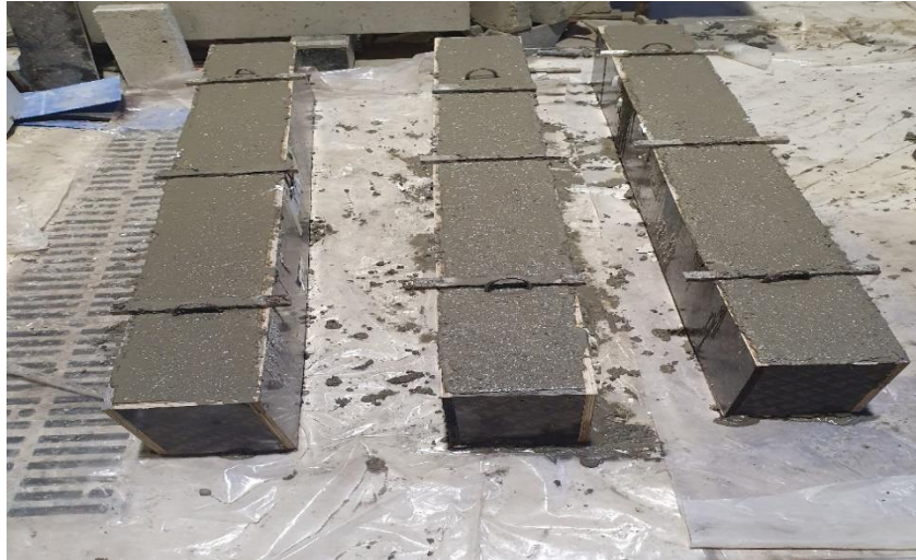
Figure 4.5 Concrete beams post casting
