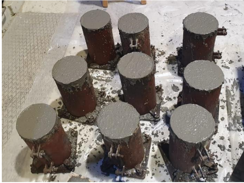
Figure 4.2 Cast concrete cylinders
