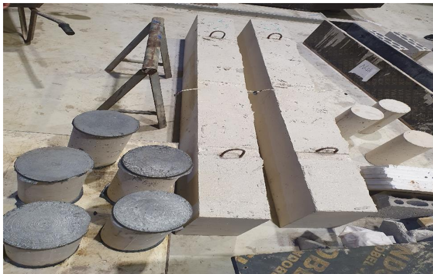
Figure 4.6 Concrete samples prior to testing
