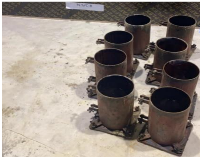
Figure 4.1 Cylindrical molds prior to concrete casting
