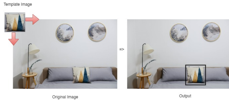
Figure 2.13: Demonstrating an Example of OpenCV Template Matching
