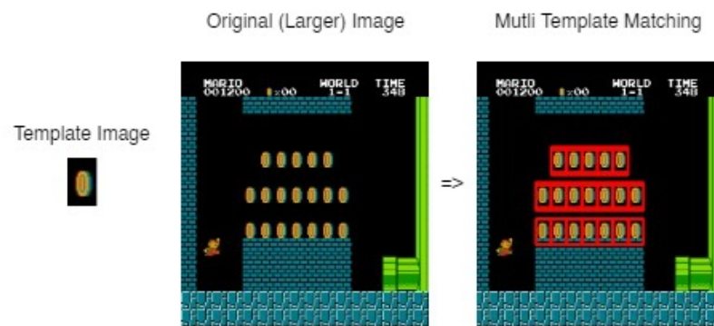
Figure 2.14: Demonstrating an Example of Multi Template Matching by OpenCV
