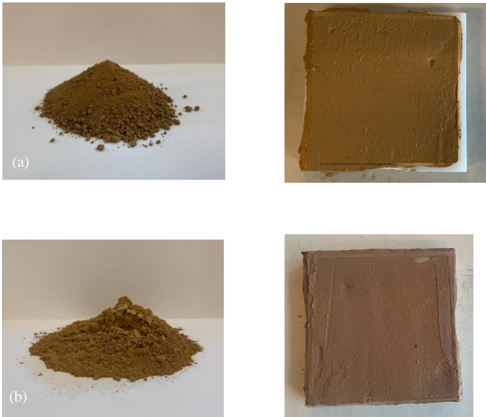
Figure 22 (a) Natural Clay with low plasticity (LPC) and (b) High Plasticity Clay (HPC)
