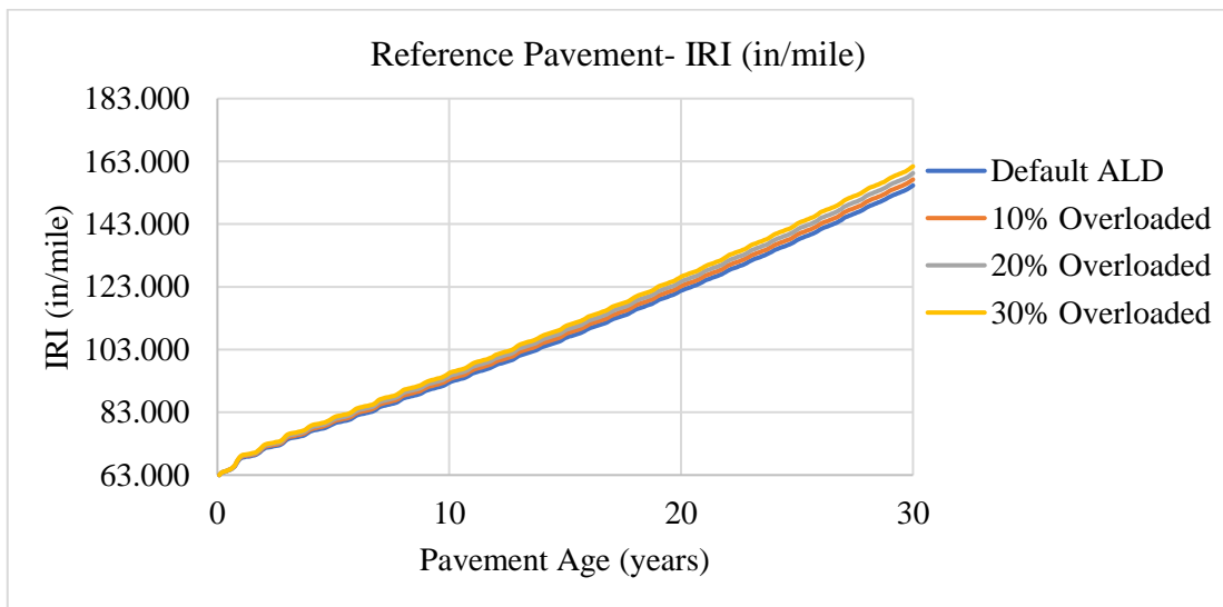
Figure 56 Predicted IRI for the Reference Pavement Structure when all Trucks are loaded based on the Default Axle Load Distribution and when Overloaded by 2) 10%, 3) 20% and 4) 30%
