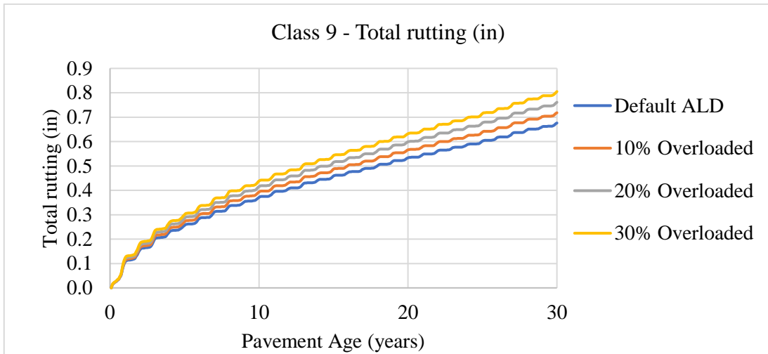
Figure 47 Predicted Total Rutting for the Reference Pavement Structure Subject to Class 9 trucks when 1) loaded based on the Default Axle Load Distribution and when Overloaded by 2) 10%, 3) 20% and 4) 30%
