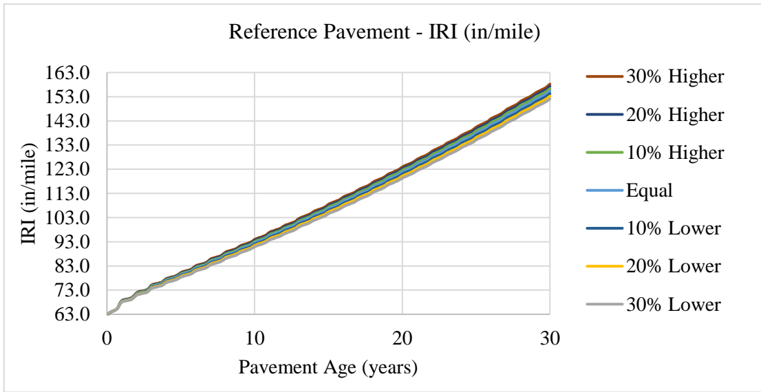
Figure 72 Predicted IRI for the Reference Pavement Considering Different Traffic Levels
