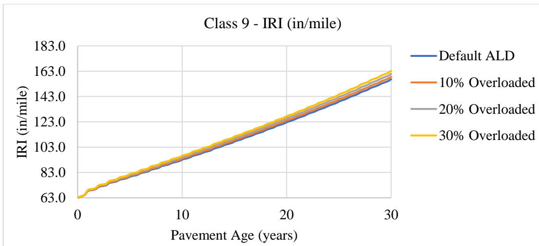
Figure 46 Predicted IRI for the Reference Pavement Structure Subject to Class 9 trucks when 1) loaded based on the Default Axle Load Distribution and when Overloaded by 2) 10%, 3) 20% and 4) 30%
