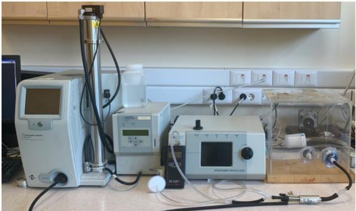
Figure 8. Scanning mobility particle sizer spectrometers setup
