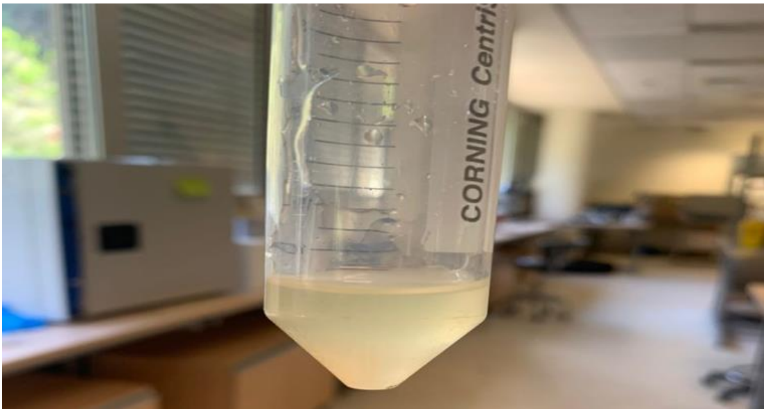
Figure 35. Dissolution of cellulose in ethylene diamine and potassium thiocyanate via vortex method
