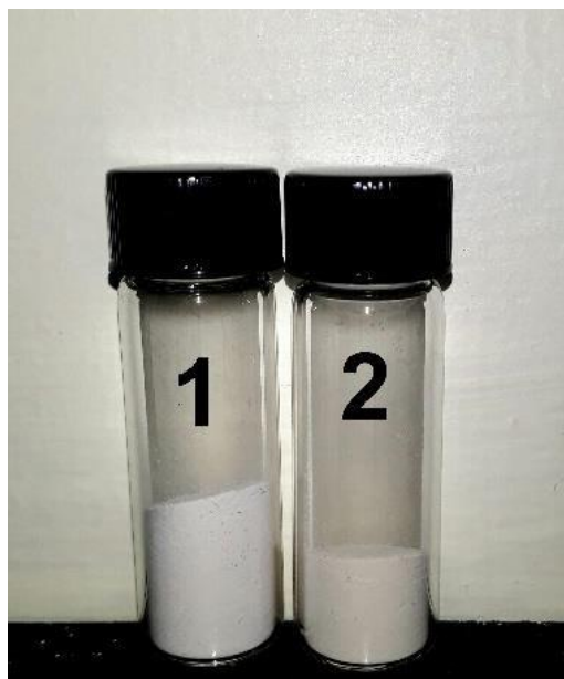
Figure 9. White dry powders obtained after the removal of the agarose gel. Left vial (1): solid crystals obtained from the uncarbonated region (pink region); right vial (2): solid crystals obtained from the carbonated regions (white bands and spherulites).
