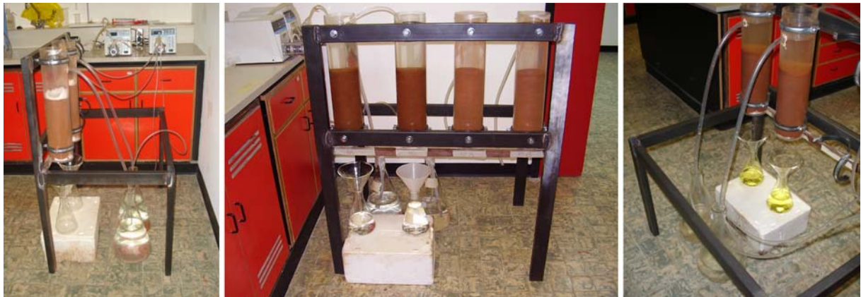
Fig. 1 a Layout of the column leaching experiments; b Illustrative photographs of laboratory sorption column experiments
