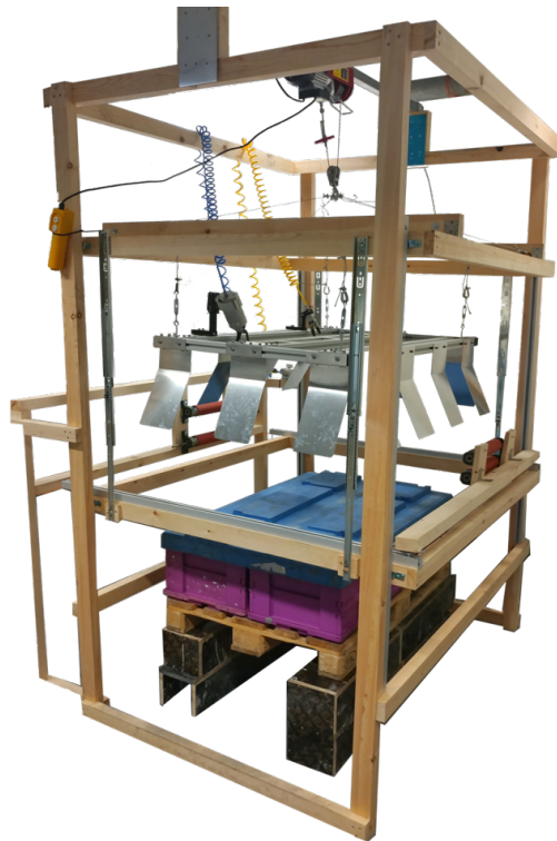
Fig. 16: Mock-up Cutting Tool Assembly (Prototype-I).
