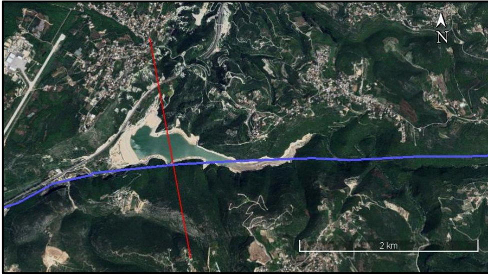
Figure 4. Aerial view of the Mseilha dam reservoir and the Batroun Fault (blue line) captured from Google Earth in April of 2020 when the dam was filled. The red line represents the location along which the 2D section in Figure 13 was taken.
