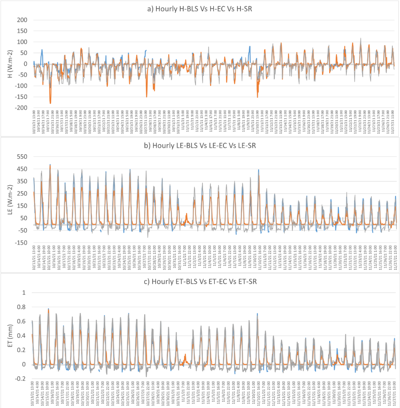
Figure 13 Intercomparison between EC, BLS and SR values for sensible heat, latent heat and evapotranspiration using hourly measurements
