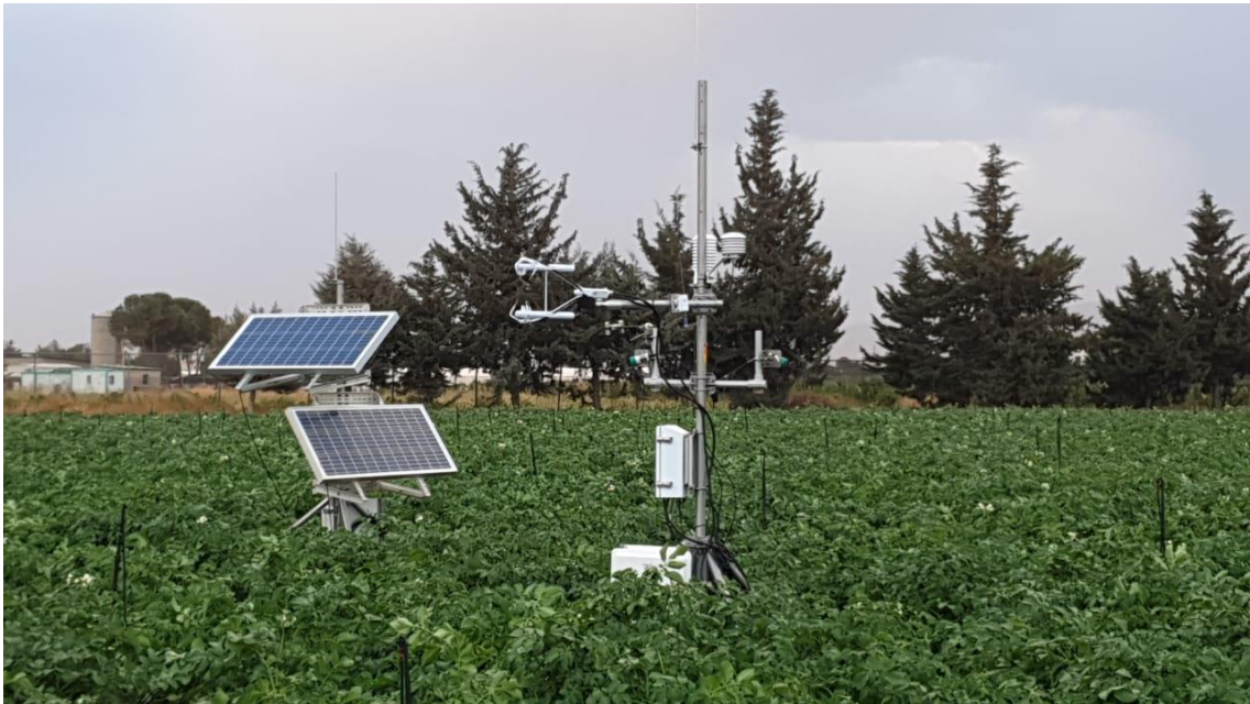
Figure 5 Eddy Covariance and Surface Renewal Systems in the Potato Field
