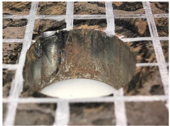
Figure 8. Hole surfaces of different bolt hole-making processes at ambient temperature for: (a) Drilled-hole, (b) Waterjet-hole, (c) Plasma-hole
