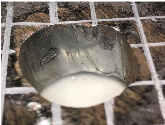
Figure 8. Hole surfaces of different bolt hole-making processes at ambient temperature for: (a) Drilled-hole, (b) Waterjet-hole, (c) Plasma-hole
