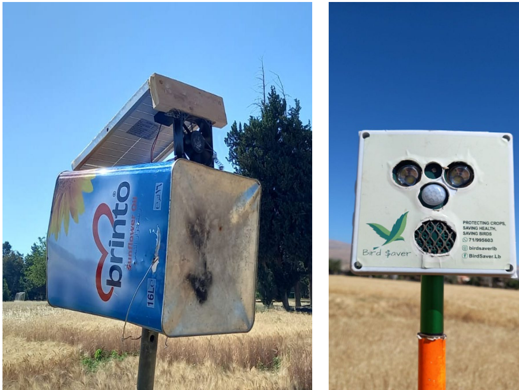
Figure 11. Images of hand-made solar bird repellent devices.
