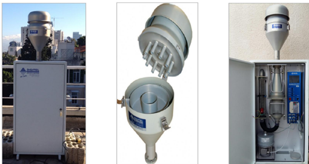
Figure 10: The high volume sampler (HVS)
