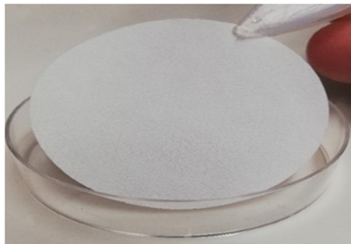
Figure 9: PTFE filter before the sampling
