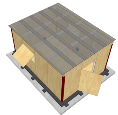
Wooden beams, corrugated panels, and poly-carbonate opening
