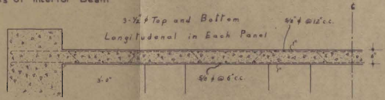
Fig 36-c Half-Cross Section Showing Slab Reinforcement
