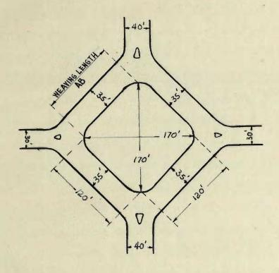
A ROUNDABOUT AT AN INTERSECTION OF A 40-FT AND A 30-FT ROAD IN THE OPEN COUNTRY
