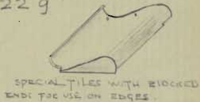
PANTILES BLOCKED GAP AT EAVES AND HIPS WITH CHIPPINGS & MORTAR
