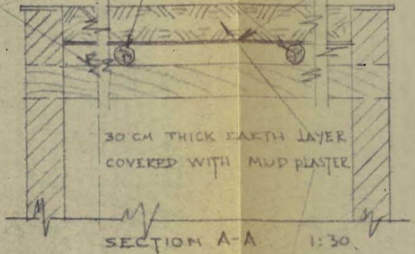
FIG I - EARTH & TIMBER ROOF
