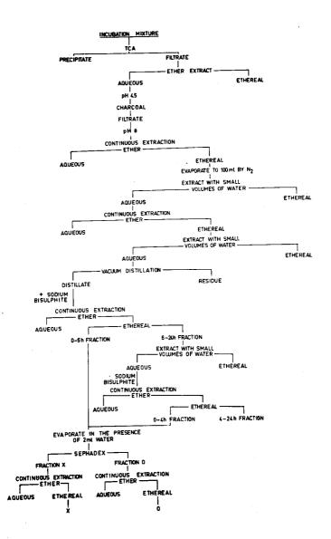
FIGURE 4. DIAGRAMMATIC SCHEME FOR THE PURIFICATION OF ACETOIN METABOLITE.
