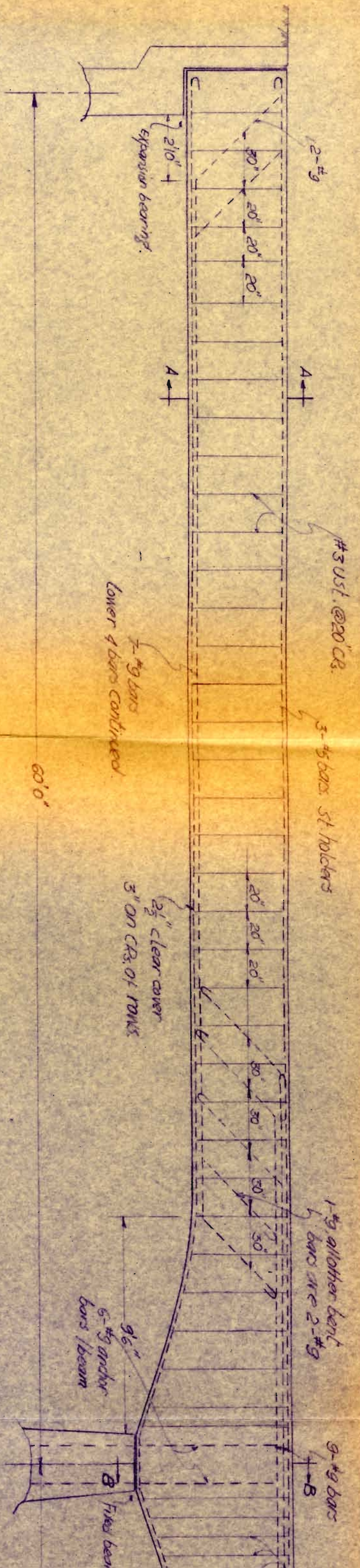
FIG. 30 LONGITUDINAL SECTION THROUGH CANTILEVER AND END SPAN
