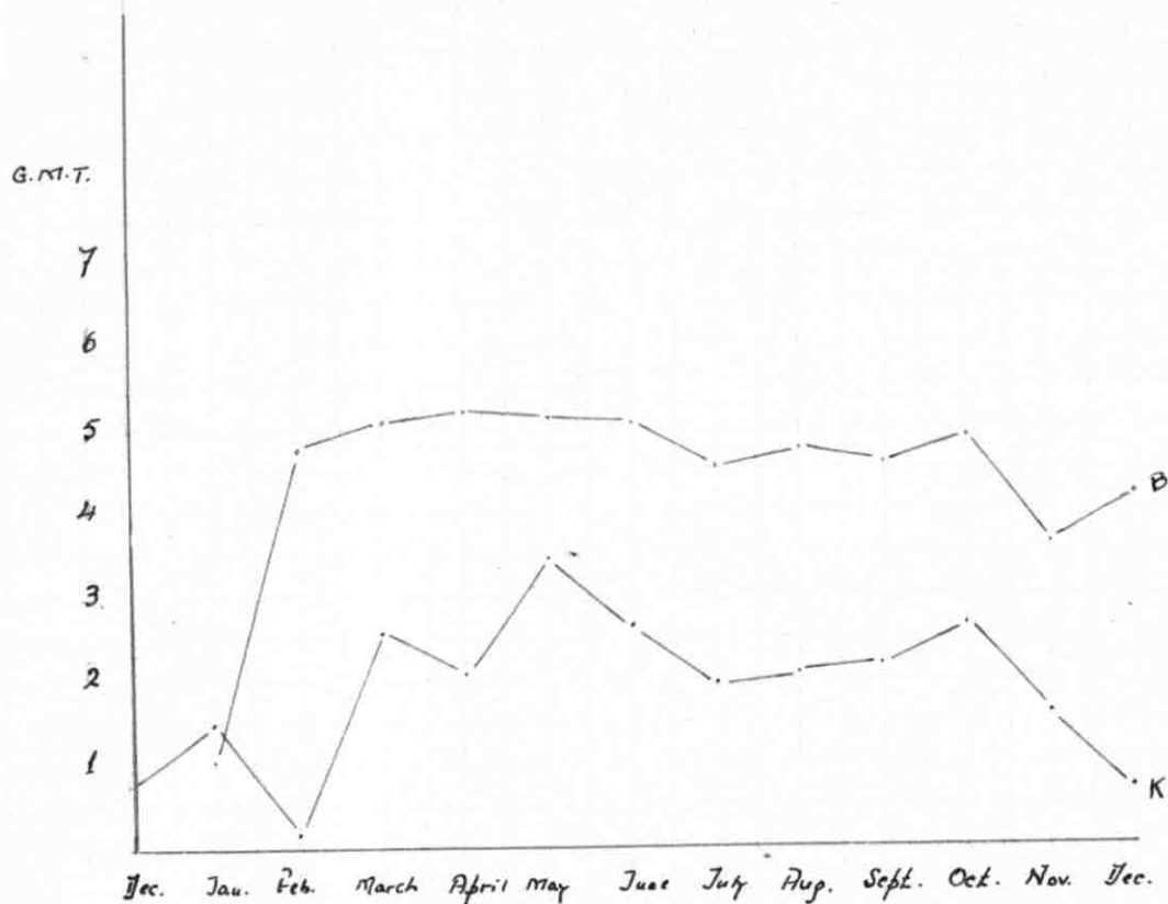
TIMES OF THE FIRST MAXIMA OF THE DIURNAL WAVES OF PRESSURE AGAINST THE MONTHS OF THE YEAR.
