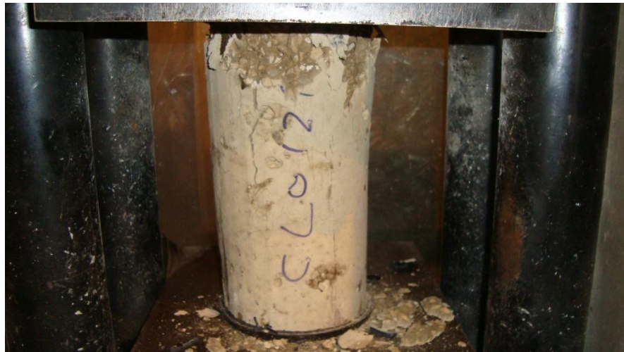
Figure 3.2. Typical Standard Cylinder (15 x 30 cm) Tested According to ASTM C39.
