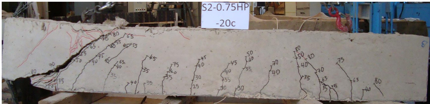
Figure A3.10. Phase 2, Shear Beam, 0.75% Hemp-20% coarse, S2-0.75% HP-20% c.
