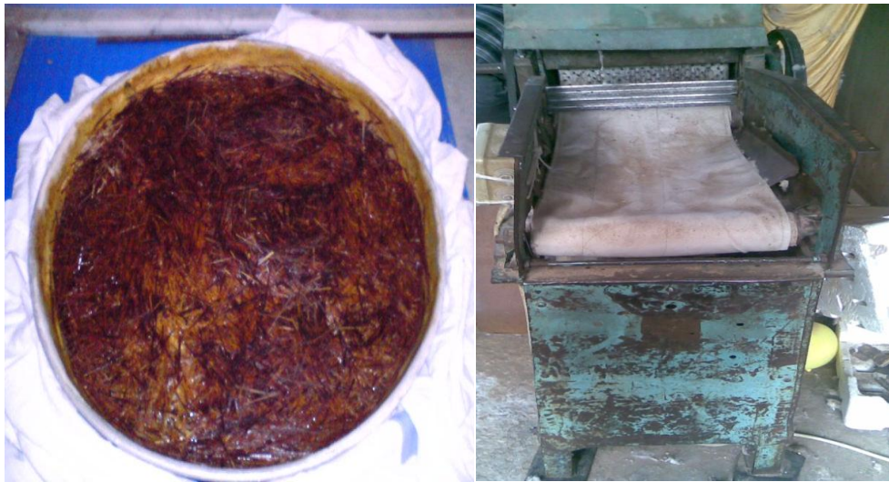
Figure A3.28. Hemp Fibers Preparation, Soaking Panel and Spreading Machine Used After Drying.
