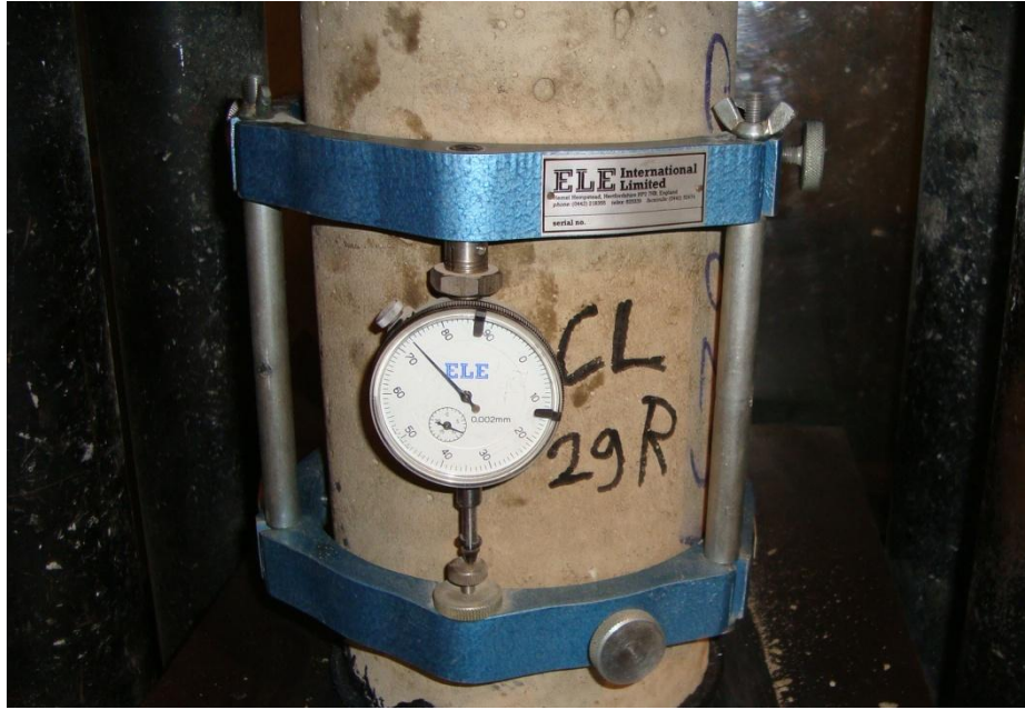
Figure 3.5. Modulus of Elasticity Test Specimen (15 x 30 cm).
