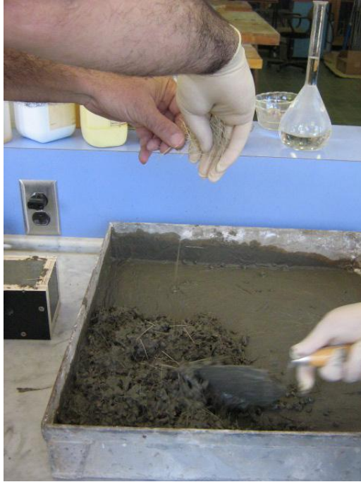
Figure A3.25. Trial Phase Mixing, Adding Palm Fibers (Wet Mix).
