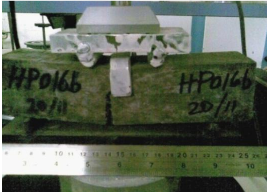
Flexure Beam (20 x 5 x 5 cm) Test
