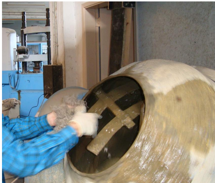
Figure A3.26. Phase 1 Mixing, Hemp Fibers Added on Wet Mix.
