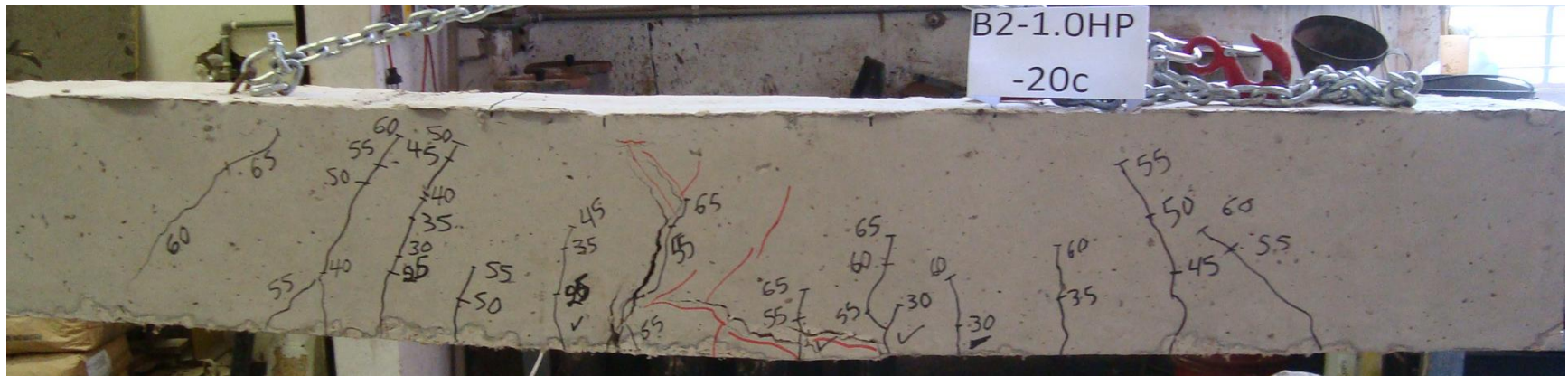
Figure A3.18. Phase 2, Bond Beam, 1%Hemp-20%coarse, B2-1%HP-20%c.
