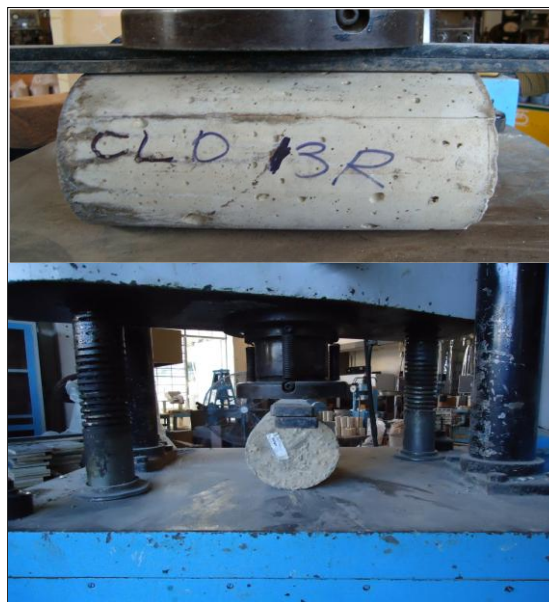
Figure 3.4. Splitting Tensile Test Specimen (15 x 30 cm), Longitudinal and Side Views of the Test Set Up.
