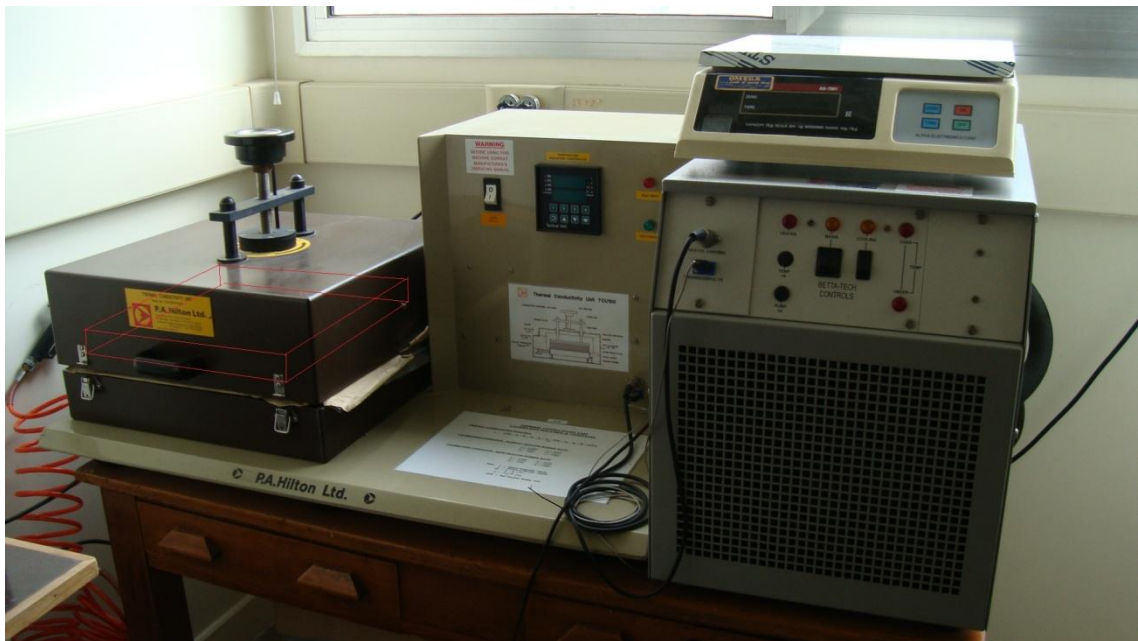
Figure 3.6. Thermal Conductivity Test Block (5 x 30 x 30 cm) Set Up.
