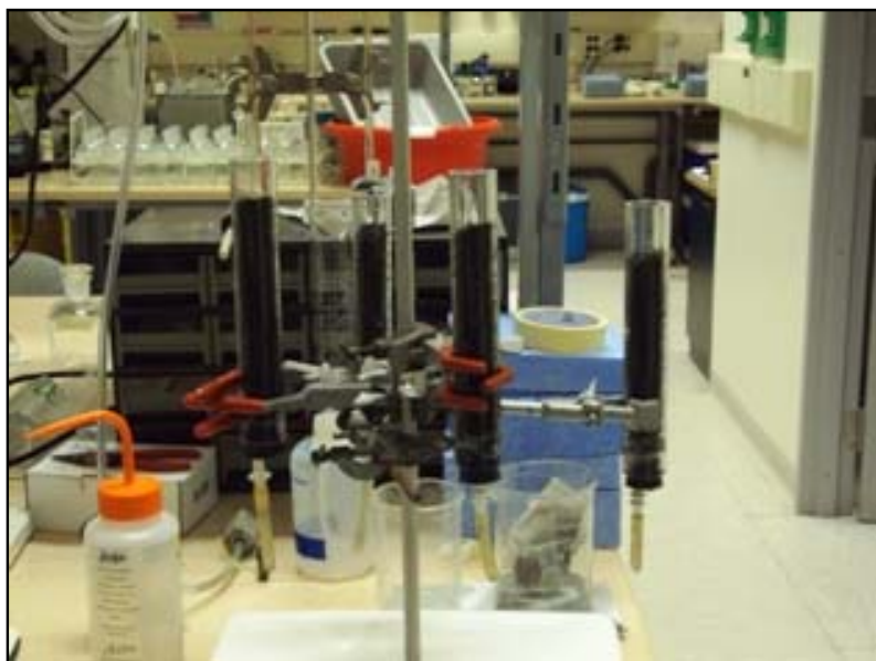
Figure 3.4 AC packed in acrylic plastic tubes
