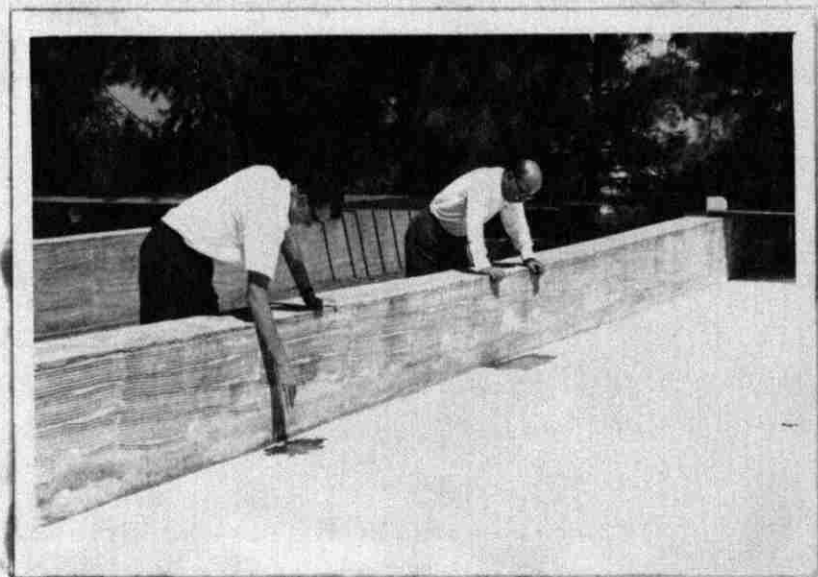
Figure 20. Openings made in Styropor layer in experimental pond for mosquito Larvae and Algae inspection. Dosage applied is 125 \text{ gm/m}^2 .
