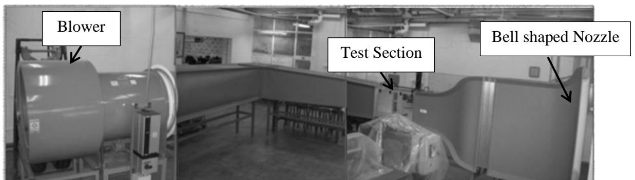
Figure 2: L-shaped wind tunnel
