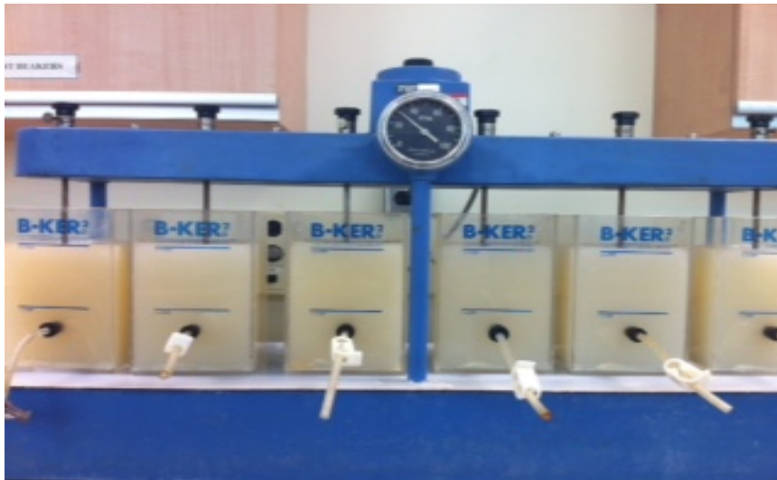
Figure 3.8 Effect of Fe spiking on color of the samples
