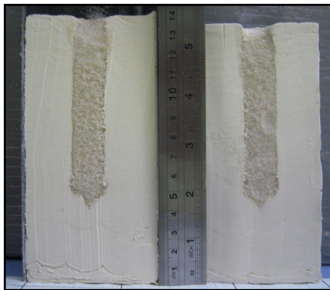
Figure 4.12. vertical cross section of Kaolin specimen with ordinary sand column of diameter 2cm and height 10.65cm after column insertion.
