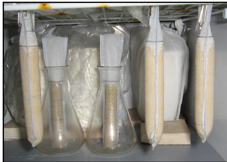
Figure 4.10. Freezing the sand columns
