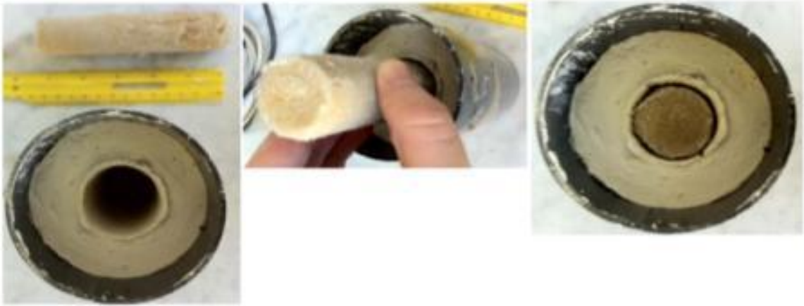
Figure 3.17. Predrilled 3-cm diameter hole, Insertion of frozen sand column in clay, and reinforced Kaolin specimen with frozen sand column
