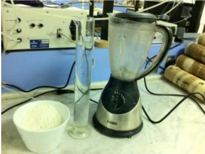
Figure 3.5. Electric Mixer for preparing Kaolin slurry
