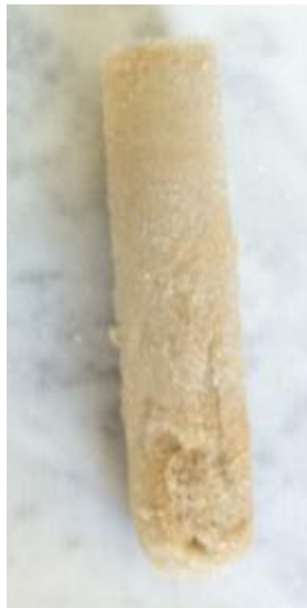
Figure 3.16. 3cm frozen sand column
