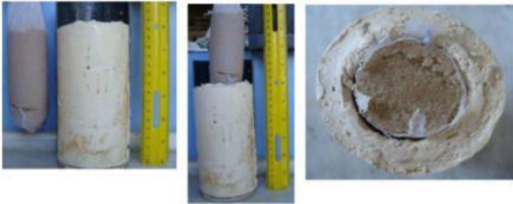
Figure 3.15. Installation of 4-cm diameter encased sand column with geotextile fabric
