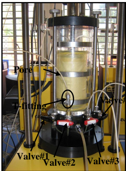
Figure 4.15. Flushing of the drains
