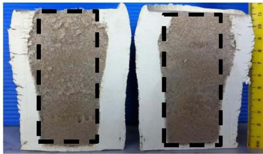
Figure 6.5 Example of external and internal modes of failure of test specimen ( H_c/H_s = 1 and A_c/A_s = 31.7\% , Ordinary).
