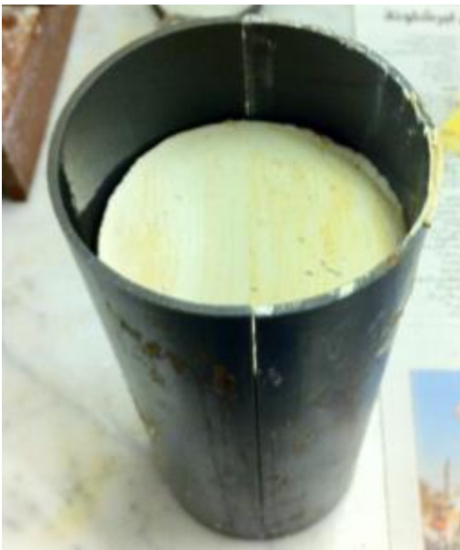
Figure 3.13. Wrapping the Kaolin specimen with PVC tubes prior to auguring
