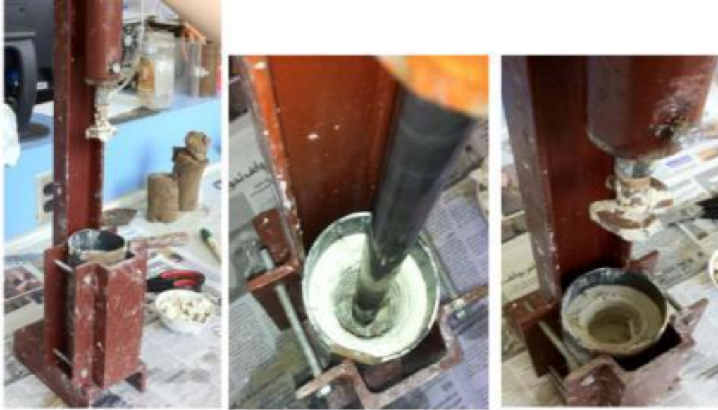
Figure 3.14. Custom fabricated auguring machine, 4cm -diameter auger, auguring of specimen by 4cm diameter augur, Removal of Kaolin material by 4 cm diameter auger
