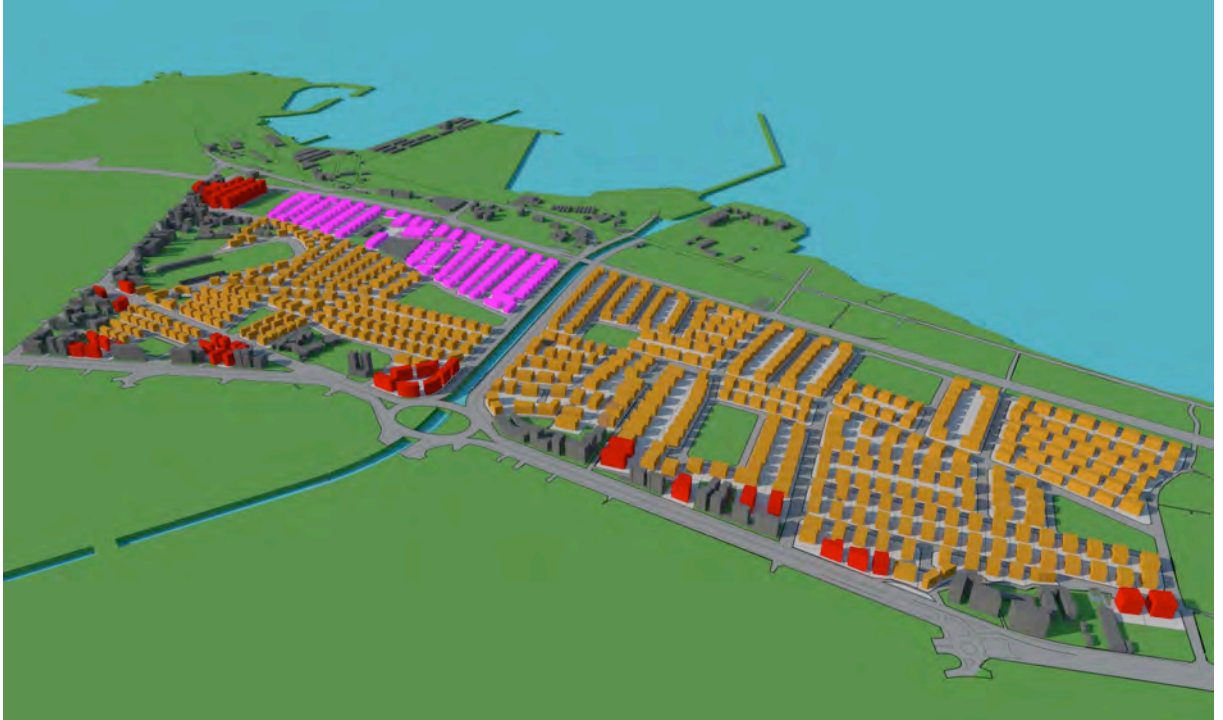
Fig. 61. Projected development: massing according to official land subdivision and zoning laws (for color code refer to Map.36). Source: by Author.
