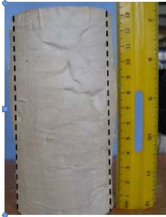
Fig..5.5 Example of external and internal modes of failure of test specimen ( H_c/H_s = 1.0 and A_c/A_s = 17.8\% encased).
