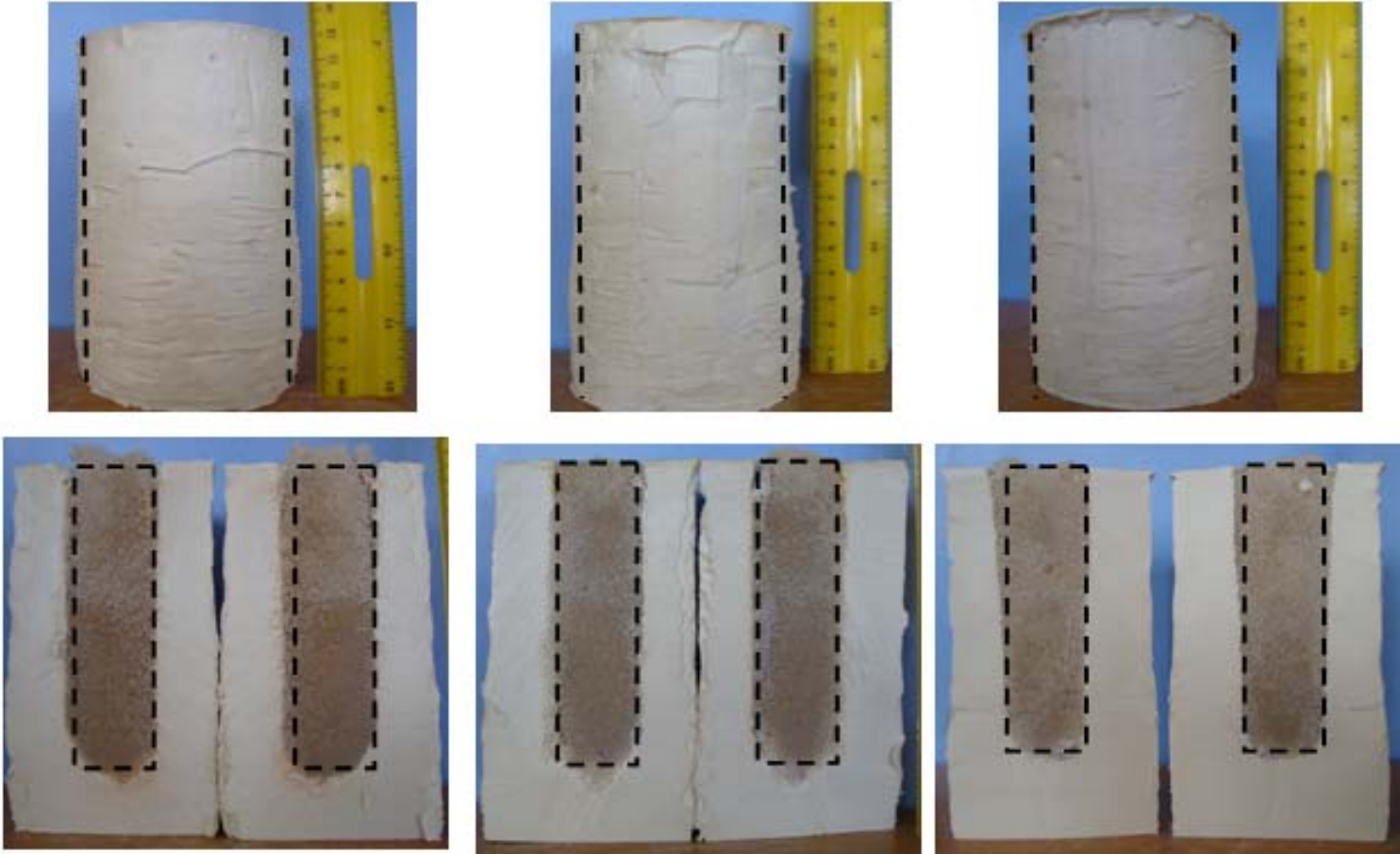
Fig.5.4 Example of external and internal modes of failure of test specimen ( H_c/H_s = 0.75 and A_c/A_s = 17.8\% encased).
