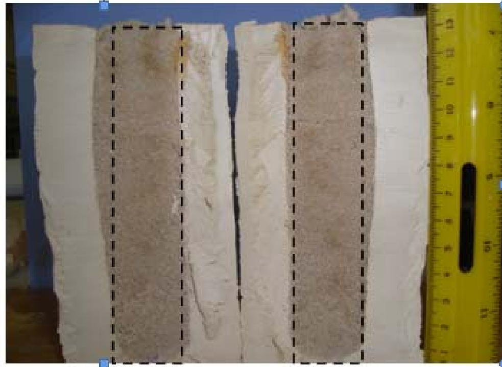
Fig..5.5 Example of external and internal modes of failure of test specimen ( H_c/H_s = 1.0 and A_c/A_s = 17.8\% encased).
