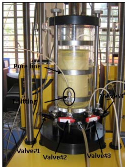
Fig. 4.15 Flushing of the drains
