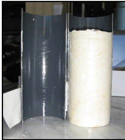
Fig. 3.20 Wrapping the Kaolin specimen with PVC tubes prior to auguring
