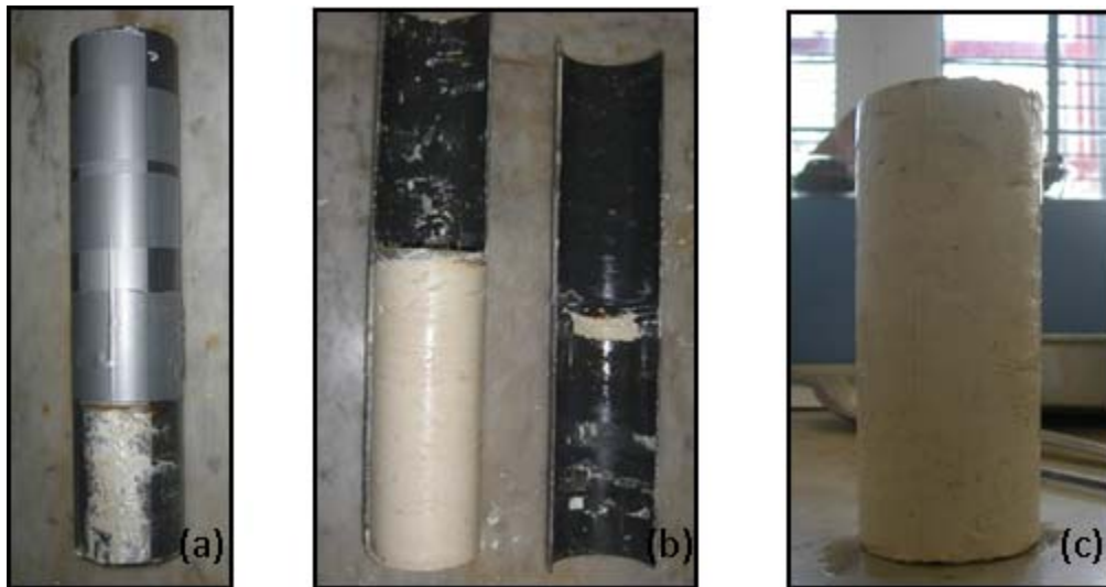
Fig. 3.17 (a) Kaolin specimen after removal from custom fabricated consolidometer, (b) dismantling of PVC pipe, and (c) Kaolin specimen after removal form PVC pipe.
