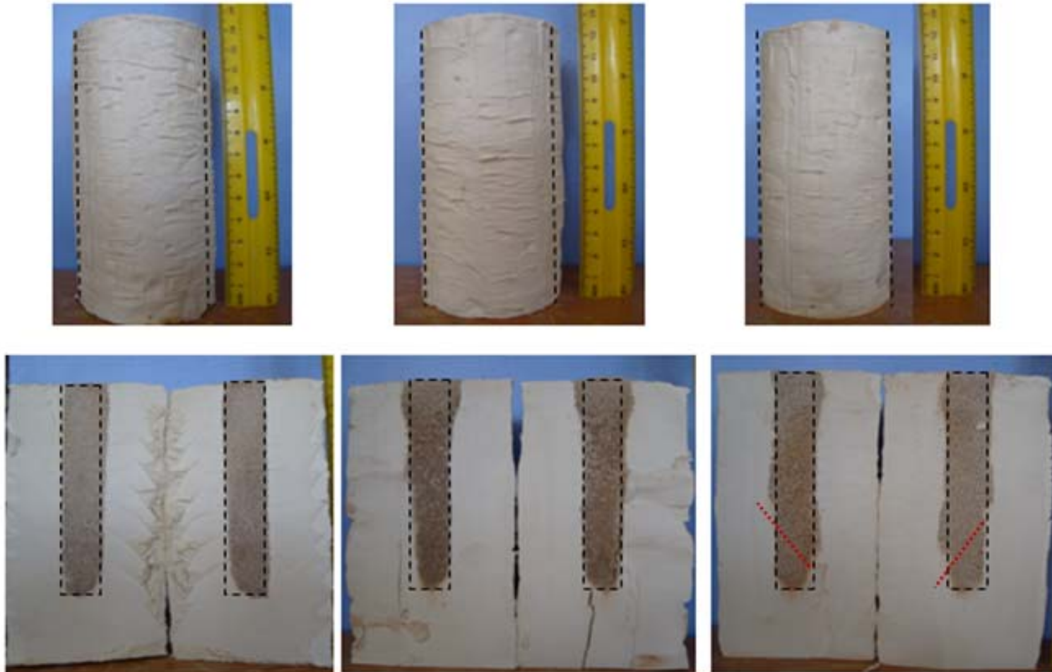
Fig.5.3 Example of external and internal modes of failure of test specimens ( H_c/H_s = 0.75 and A_c/A_s = 7.9\% , ordinary)
