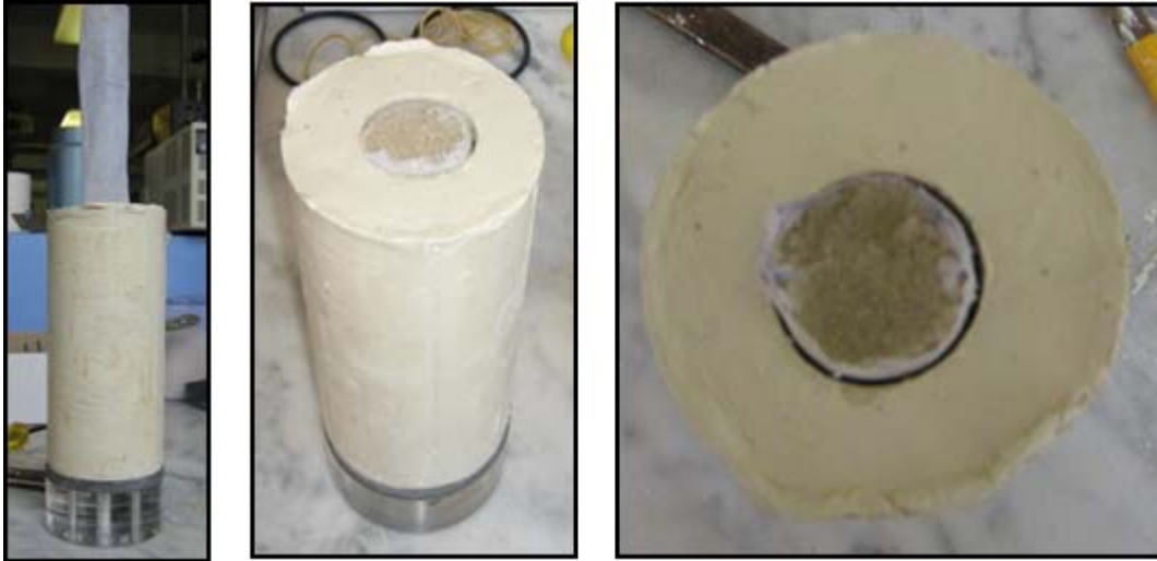
Fig. 3.23 Installation of 3-cm diameter encased sand column with geotextile fabric
