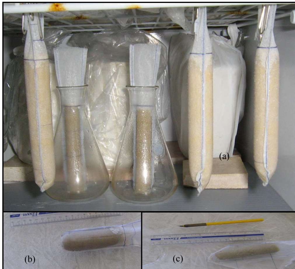
Fig. 3.24 (a) Freezing the sand columns (b) and (c) removal of geotextile fabric
