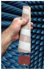
Fig. 6. (a) Z-folding progression scheme. (b) Implementation of the folding process on the fabricated prototype.
