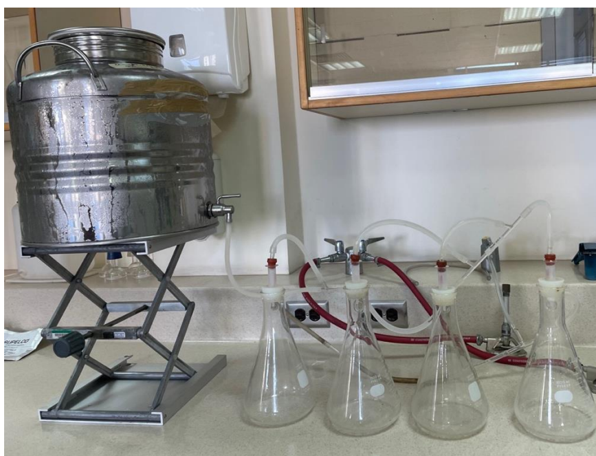
Figure 3 Water Extraction Apparatus for the 60L water samples
