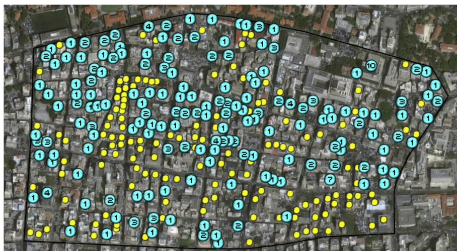
Fig. 1. The Hamra area showing the 588 buildings that were surveyed. 258 generators were identified in 168 buildings (blue circles) and missing information is for the remaining 142 buildings (yellow circles). (For interpretation of the references to colour in this figure legend, the reader is referred to the Web version of this article.)
