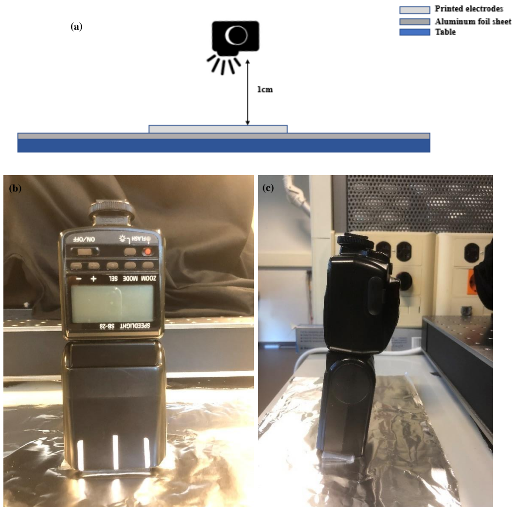
Figure 16. Flash sintering set-up using a camera flash. (a)Schematic diagram of the set-up (b)front view of the set up with Nikon Speedlight SB-28 (c)Lateral view with sample
