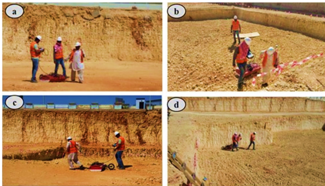
Fig. 4 Field GPR data acquisition a–d in one of the investigated sites
