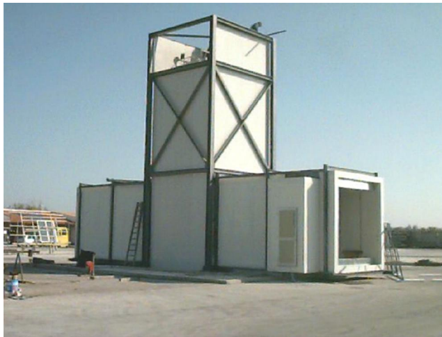
Figure 2. Passive downdraft evaporative cooling experimental test facility [40].
