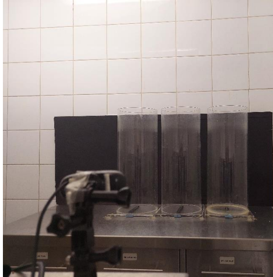
Figure 6 Forced Swim test Setup . Each cylinder was filled with water and the rats were left to swim for 10 minutes per session. Rats were video recorded while swimming using the camera shown in the figure.
