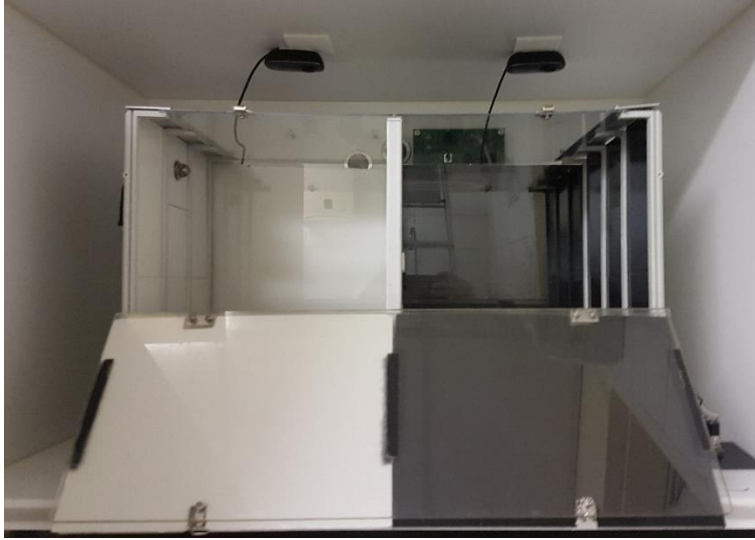
Figure 4 Light dark box apparatus. The right chamber is dark with no illumination and black walls while the left chamber is lit with bright illumination and white walls. Two cameras are placed above each box for video recording.
