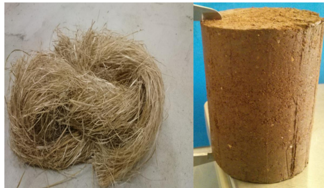
Fig. 1. Bundle of hemp fibers and typical compacted soil specimen. (Images by Shadi Najjar.)
