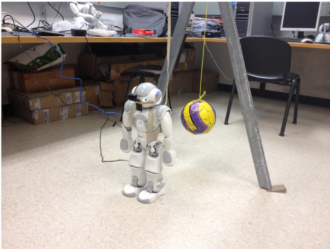
Fig. 7. The whole system is shown in this figure. The humanoid and camera are connected to the laptop running C++ and python code.
