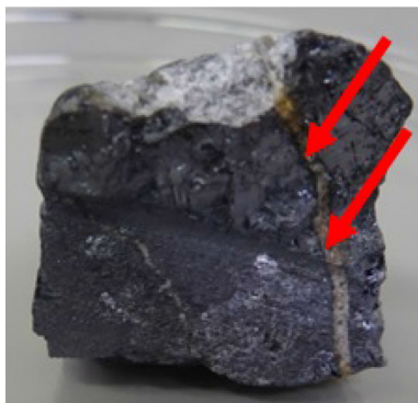
Fig. 4 Longitudinal cross-section of a treated galena rock (drilled at the center) and acidized with 2 M sulfuric acid. The rock is essentially compact and homogeneous; rare canals (indicated by the red arrows) may be present in the original sample
