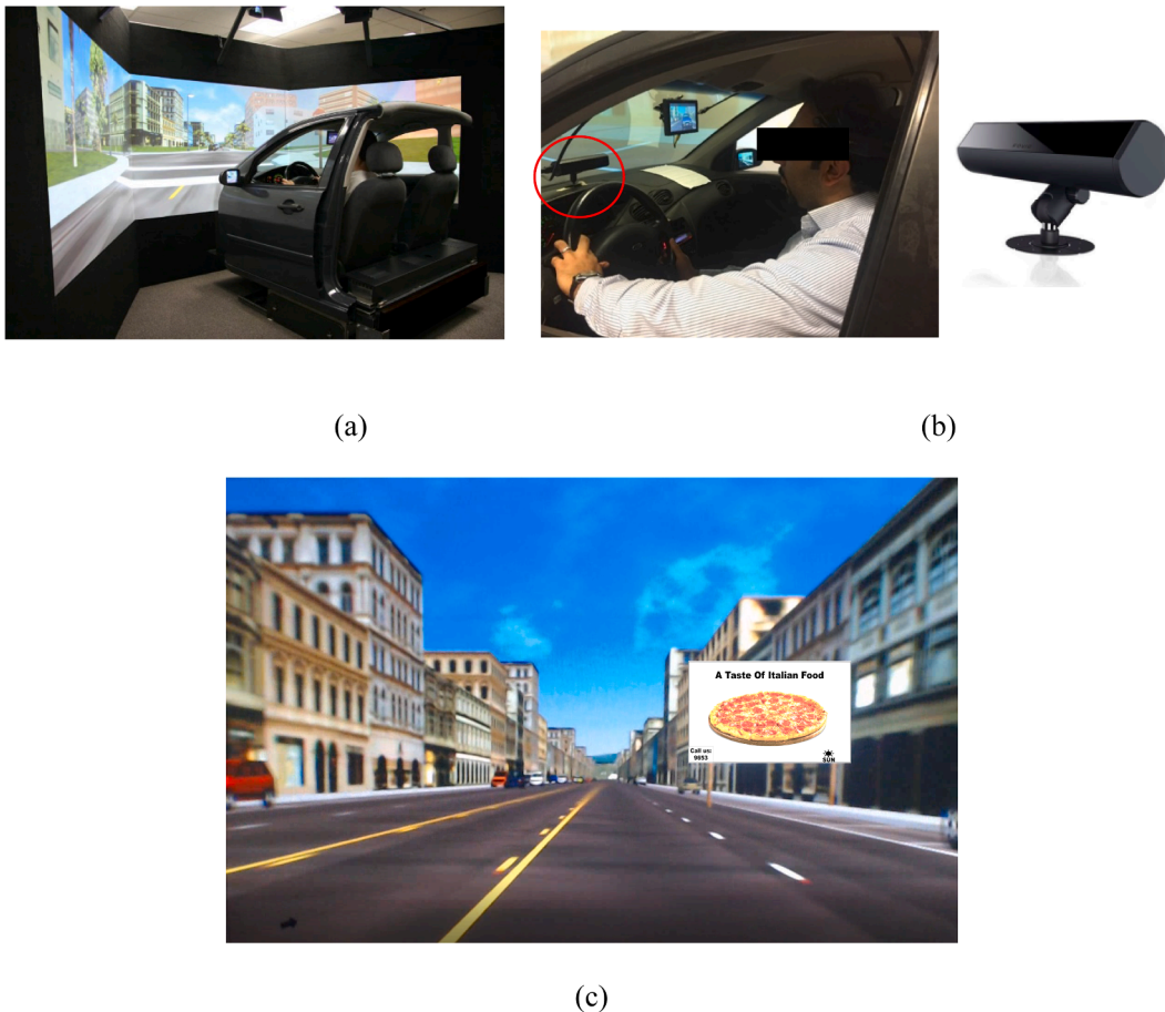
Fig. 1. (a) The experimental setup with the DriveSafety™ Driving Simulation System, (b) the Fovio Eye Tracker from Eye Tracker Incorporation, and (c) a view from the car, showing a DBA.
